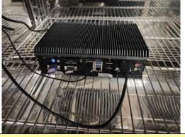
4. High Temperature and High Humidity Test / Low Temperature Test
